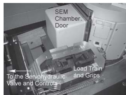
Fig. 4 Servohydraulic load frame that can be inserted into a specially equipped SEM for in situ experiments. The interaction of the unique plasma sprayed microstructure with the applied load can be viewed directly using this equipment.
